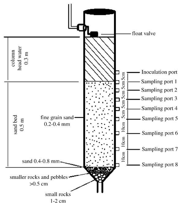
**Fig. 1** – Detailed schematic representation of an individual slow sand filter column. Six replicate filters were constructed and the resulting design and set-up of the columns allowed a continuous flow of microcystin LR-dosed dam water to pass through the sand beds.
