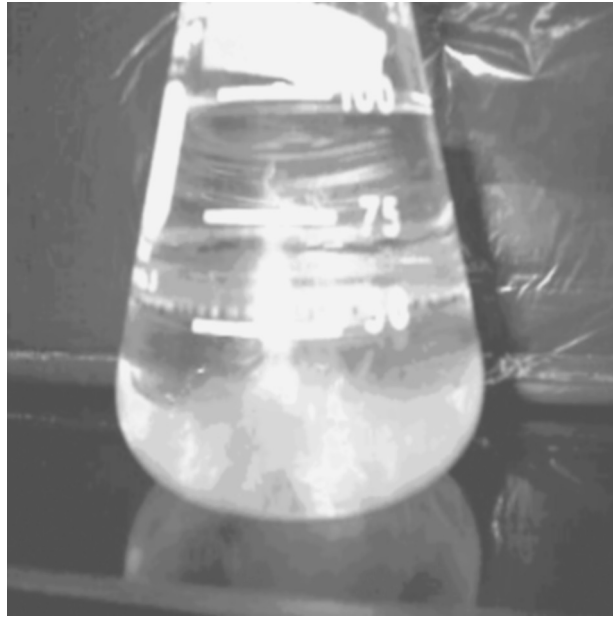
Figure 6. Polymer film formation at the interface of oil and water phases in a canola oil-contaminated wastewater sample, 2 \times .
