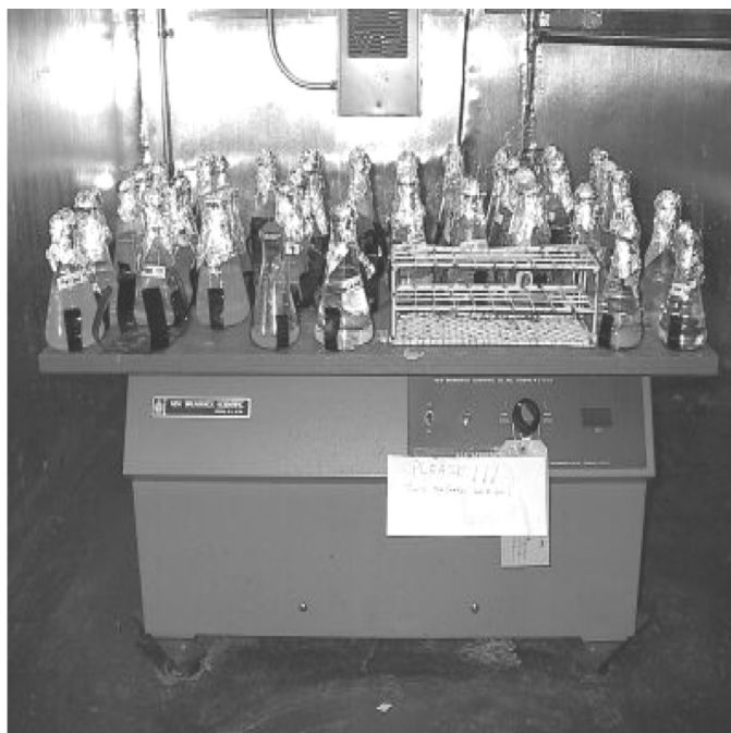
Figure 1. Oil-contaminated samples kept on a shaker in an incubation room at 27°C.
